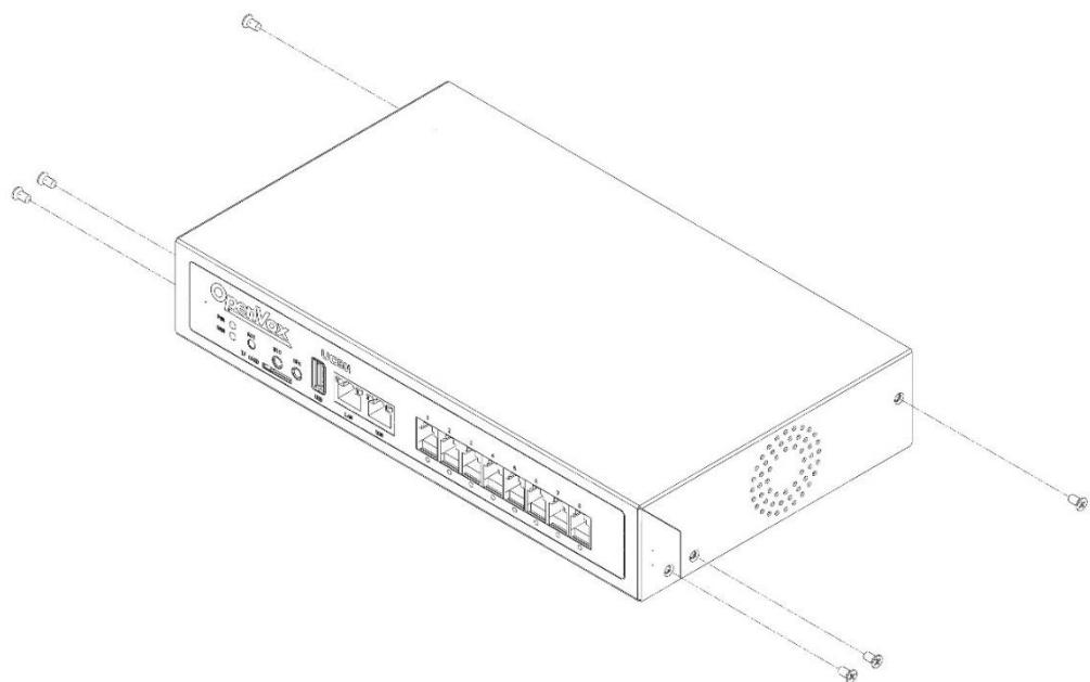
2. Remove the upper casing in the direction shown in picture.
