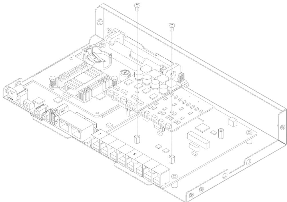
Remove the screw and install the module(②+③mode).
