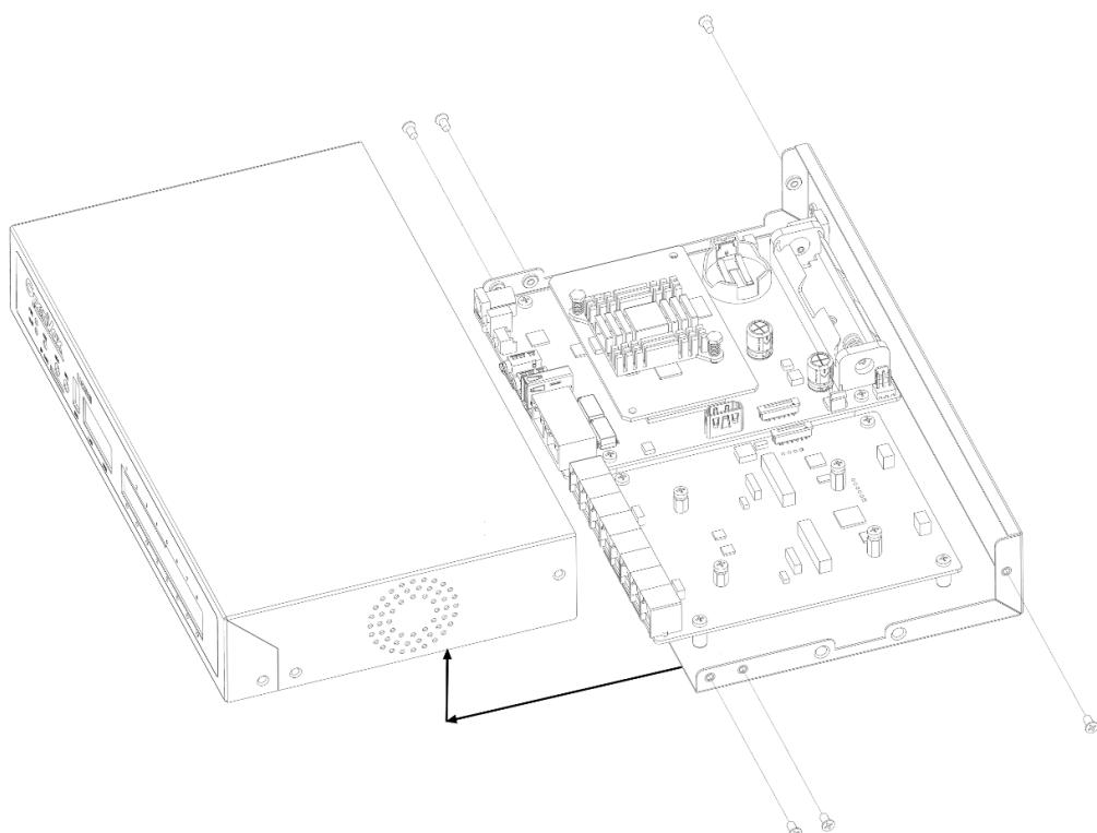
3. Below is the top view of the inside of the chassis, and the right side is the module installation area. The upper area is for the FXO-100/FXS-100 module and the lower area is for the FXO-400/FXS-400 module. It should be noted that the module cannot be installed on the left or right side at the same time, only supports ①+②, ③+④, ①+④, ②+③.
