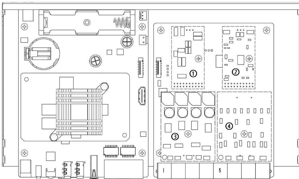
3. Remove the screw and install the module(③+④mode).
